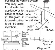
Note: Apply sealant "Mill-Pac" to inner pipe and high temperature silicone sealant to outer pipe on every twistlock joint.
